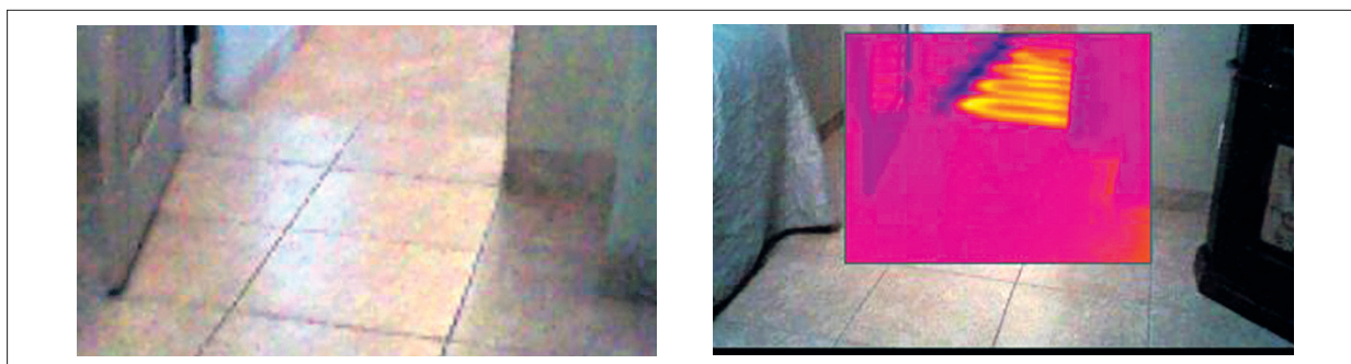
Two examples of problem-finding via infrared inspection, with naked-eye images on the left and infrared-camera images on the right. Above, the camera reveals cold-air infiltration where a viga penetrates a wall. Bottom, the radiant-heating zone in foreground appears to be nonfunctional.
