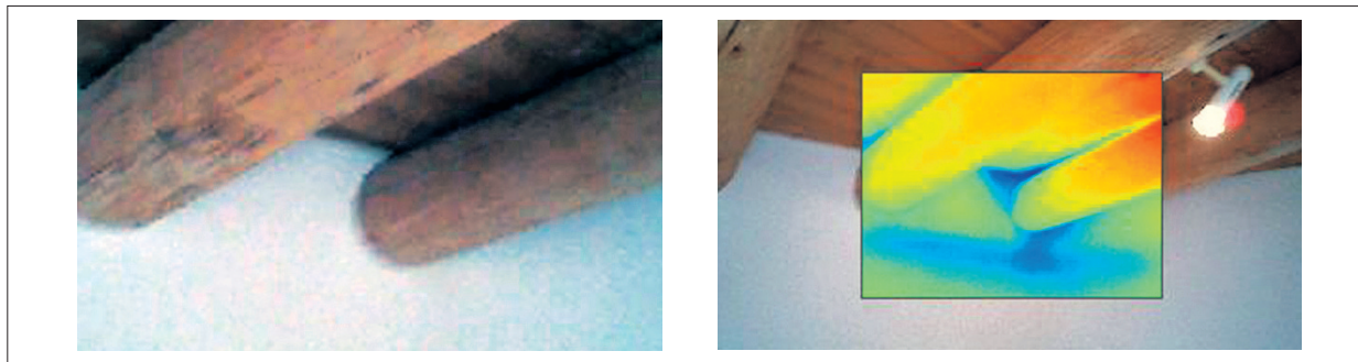
Two examples of problem-finding via infrared inspection, with naked-eye images on the left and infrared-camera images on the right. Above, the camera reveals cold-air infiltration where a viga penetrates a wall. Bottom, the radiant-heating zone in foreground appears to be nonfunctional.
